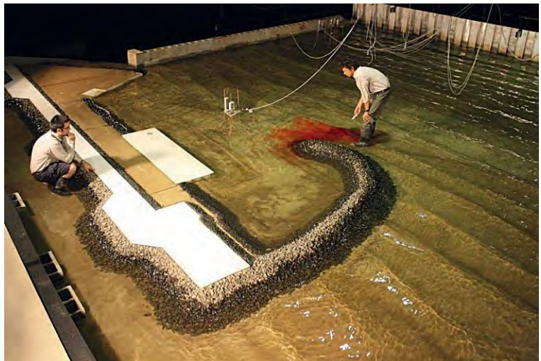
Laboratory model of Barrow Island harbour SOURCE: Water Research Laboratory, UNSW
