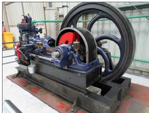
Crossley Bros. Ltd., Manchester, UK. 1924 diesel engine with a single horizontal cylinder, used for teaching engineering students at Melbourne University.
