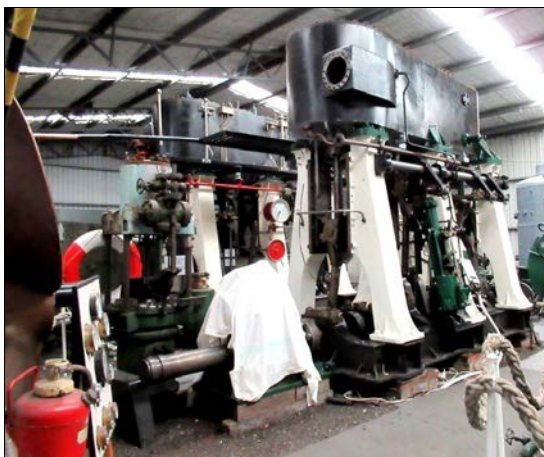
The main engines of the former twin-screw, sea-going, steam tug Lyttelton 2, built by Renfrew & Co Ltd, Renfrew, Scotland in 1939. Part of one of the twin screws is visible at left.
