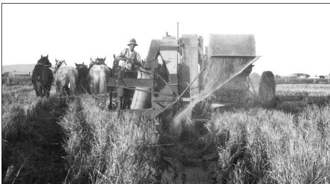
Bagging wheat from a horse-drawn Sunshine Harvester in the 1930s. This is probably an experimental rig with an engine to drive the harvester machinery (note the exhaust pipe). Ph: F/H Collection © M. Doring.
