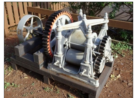
A small "Cuban" Mill, used for crushing samples of sugar cane for testing the juice to see whether the cane was ready for harvesting. Photo: KB.
