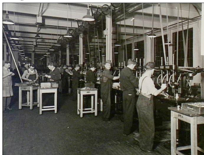
Making Bren Guns, SAF, May 1940. This early production line in the drilling section was driven by flat belts from overhead lineshafts. Photo No. 001759 from AWM.
