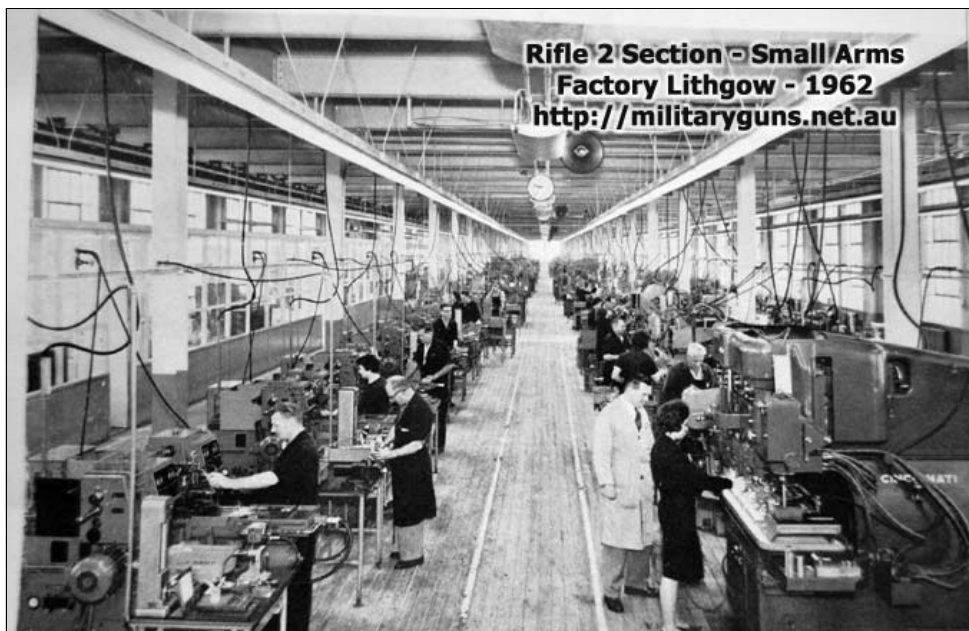
The Rifle section at SAF in one of the new buildings, long after WW2. Note these machines have individual electric motors - no lineshafting. Note also the women operators. Photo details - see top right.
