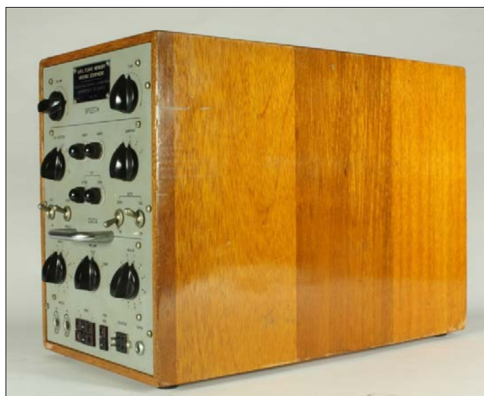
Ground Playback or Decoding Unit for separating audio & instrument data from the recorded signal. Part of the Mk.2 "ARL Flight Memory" prototype "Black Box" flight recorder, developed in 1961 - 1962.
