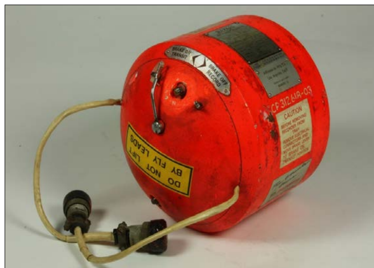
Type 1190, 'Red Egg' Recycling Wire Flight Recorder, developed by S. Davall & Sons Ltd, Greenford, London, England, from the 'ARL Flight Memory' prototype, c1967. Photo: Matthew Churchward, Museums Victoria.
