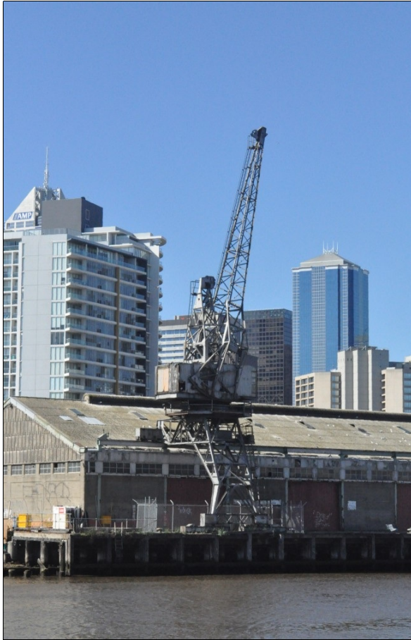
The Malcolm Moore semi-portal crane photographed in 2011 at the west end of the North Wharf Cargo Shed.
