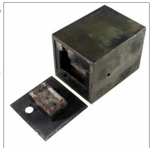
Fireproof case used in the fire testing of the Mk.1 “ARL Flight Memory” prototype “Black Box” flight recorder, circa 1958. Photo source: Museums Victoria.
