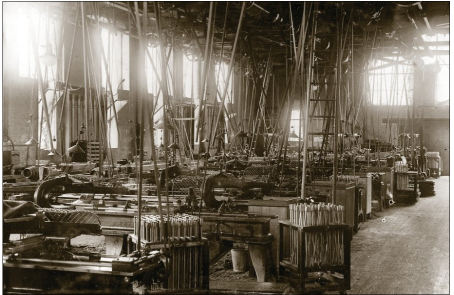
Lithgow SAF Machine Shop, Boring & Rifle Barrels Section in 1914. From the SAF Museum Archives. As was typical at the time, machines did not have individual electric motors, but were powered by flat leather belts run from overhead pulleys on lineshafts.
